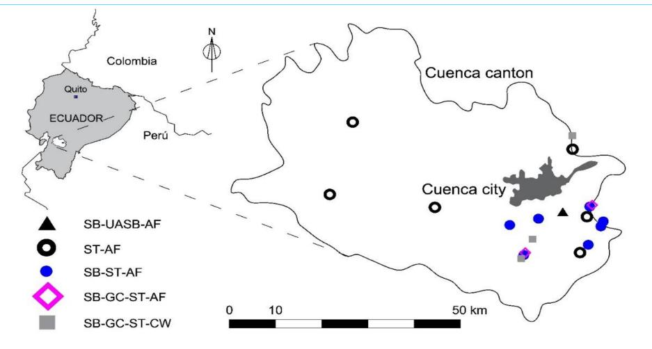
SB: Screen Bars; GC: Grit Chamber; SP: Septic Tank; AF: Anaerobic Filter; CW: Constructed Wetland; UASB: Upflow anaerobic sludge blanket
